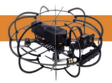
The Stereo2 is fitted with a lighting system specifically designed for inspections in confined spaces.
