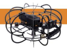
Industrial environments rhymes with dust. Once in suspension, lifted off the surfaces by the movement of the propellers, an opaque cloud can quickly appear. The Stereo2's indirect lighting system gives it a perfect view of the environment in these conditions, so the pilot can easily complete his inspection.
